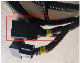
Note: The working time of the preheating plug is controlled by the engine ECU. Firstly, confirm whether the preheating plug is correctly connected during the wiring process; Secondly, whether the preheating relay is working properly.
