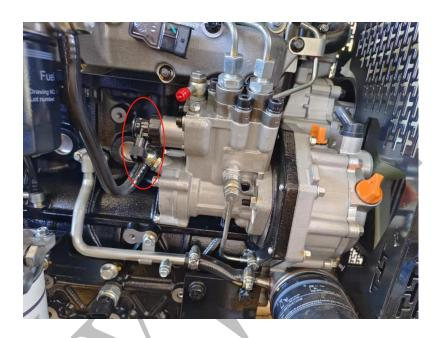
Note: For the 4F series, the ECU only controls the oil pump oil quantity, which is the transmission control signal at the position indicated in the figure.
