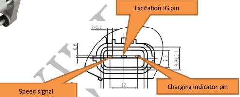
Note: The land generator set has provided excitation wires on the engine harness; The generator is not self-excited, and the IG signal is normally energized in the ON position.
