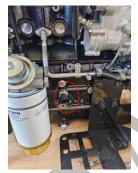
Oil pressure sensor: VDO 10Bar
