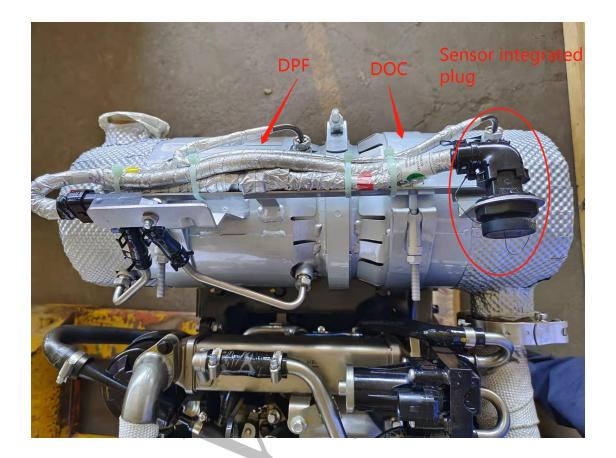
The post-treatment system is an exhaust gas treatment system that achieves emission requirements by adsorbing impurities in the exhaust gas. The post-processing device includes three sensors: DOC exhaust temperature sensor, DPF exhaust temperature sensor, and differential pressure sensor.
